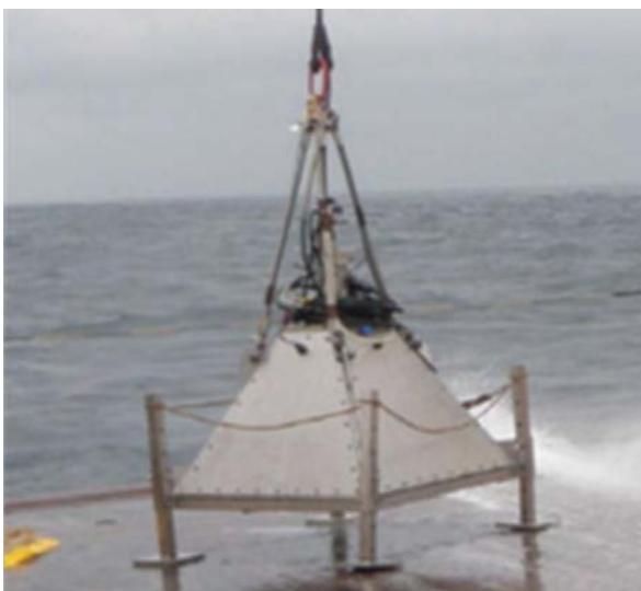
Fig 2.3 Seabed imaging camera system that uses a freshwater lens to reduce interference from suspended solids in the water column. From MES Ltd.
