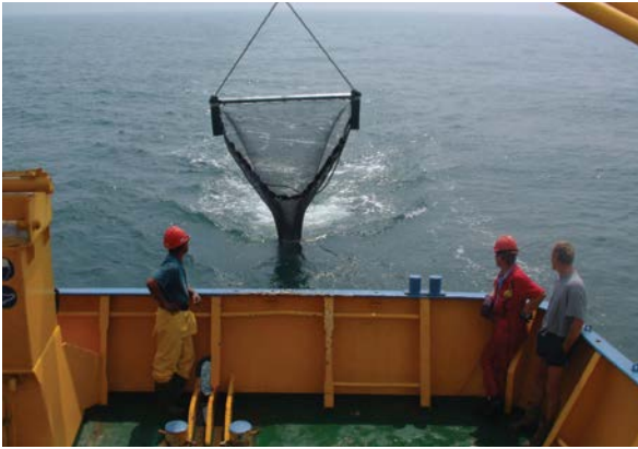
Fig 2.6 Scientific Beam trawl used for sampling epibenthic fauna. Courtesy of MES Ltd.
