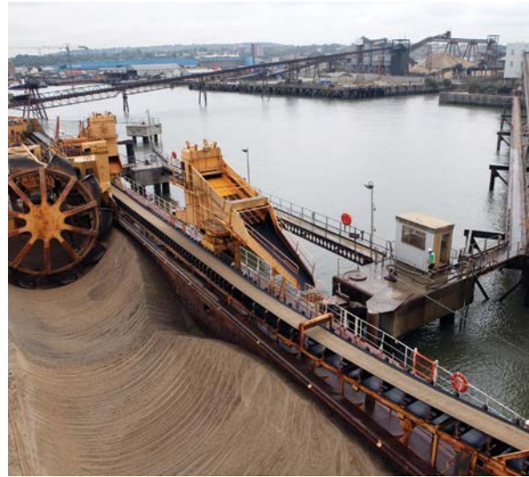
Fig 1.12 Dredger unloading its cargo of marine aggregates at an aggregate wharf using a bucket wheel. Courtesy of Mark Russell of BMAPA.
