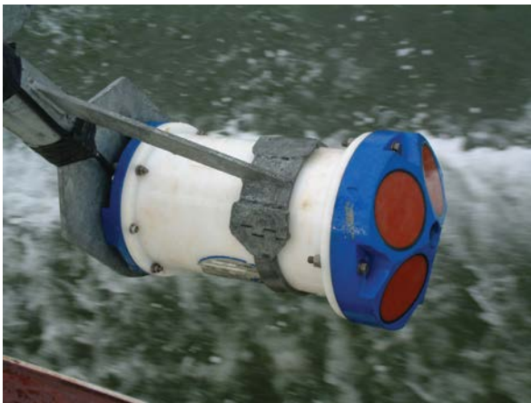
Fig 5.8 Acoustic Doppler Current Profiler (ADCP), © MES Ltd.
