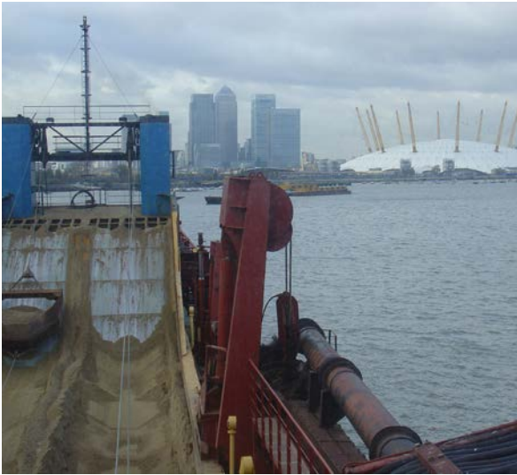
Fig 1.11 Dredger unloading its cargo of marine aggregates close to the centre of London using scraper buckets. Courtesy of Mark Russell of BMAPA.
