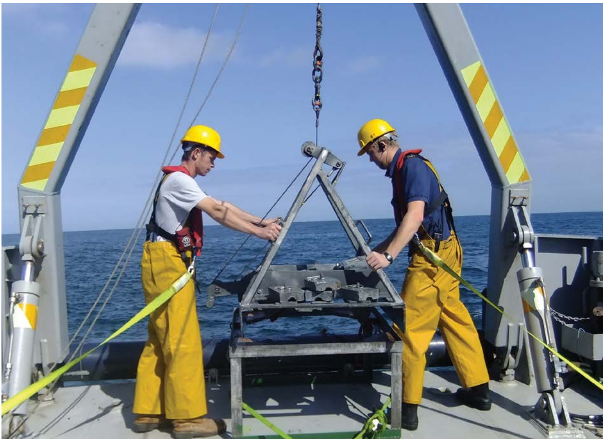
Fig 2.8 Mini-Hamon grab which is widely used to obtain seabed samples from mixed sands and gravels. Courtesy of EMU Ltd.
