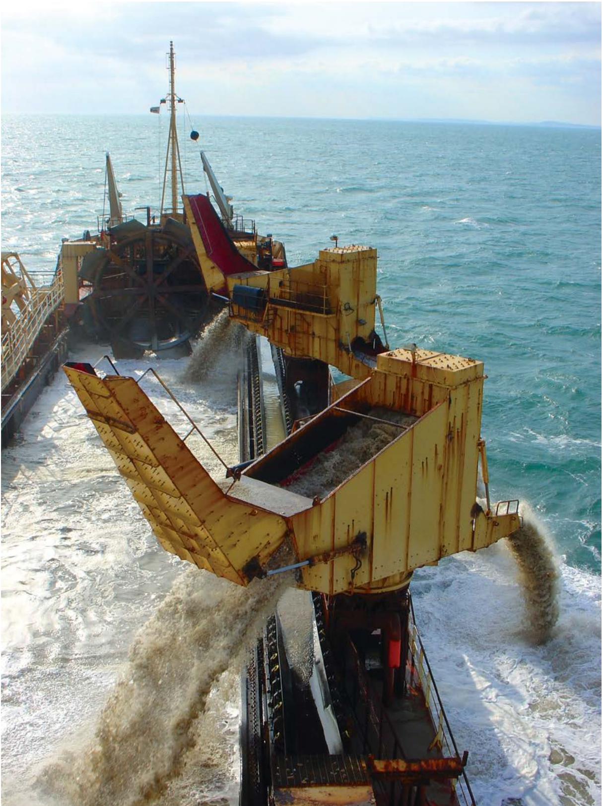
Fig 5.17 Screened and overflow sediment returned to the water column during dredge screening processes at sea (courtesy of BMAPA).
