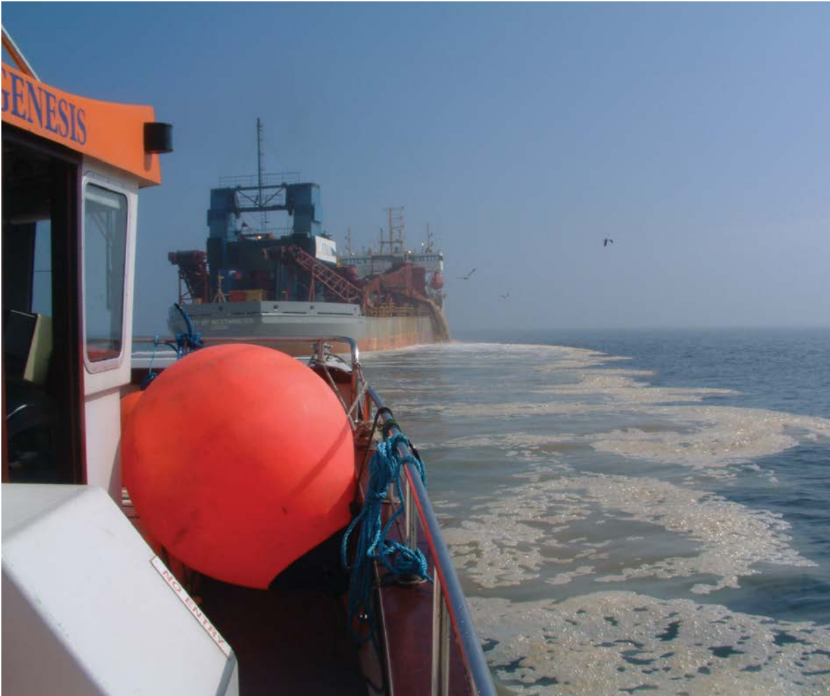
Fig 5.16 Sediment plume created by the release of sediment back into the water column, © MES Ltd.
