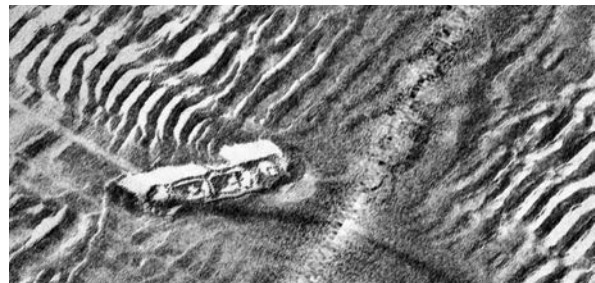
Fig 5.4 Side-scan sonar image showing ripple marks in the sand and a seabed wreck. Courtesy of Cefas.
