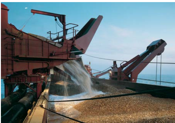
Fig 1.8 Dredged material being transferred into the hold of the vessel. Sourced from BMAPA.
