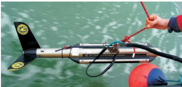
Fig 5.3 Side-scan sonar equipment.
