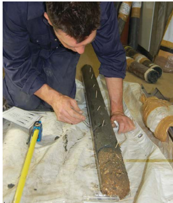
Fig 4.10 Analysis of a sediment vibrocore sample from the Humber REC. Courtesy of the University of Birmingham.
