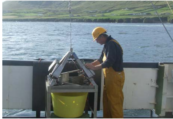
Fig 2.7 Standard 0.1m 2 Day grab used for sampling soft sediments. Courtesy of Dr John Coppock.
