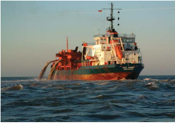
Fig 1.9 Photograph of the Arco Humber dredger showing reject chutes and overspill, © MES Ltd.
