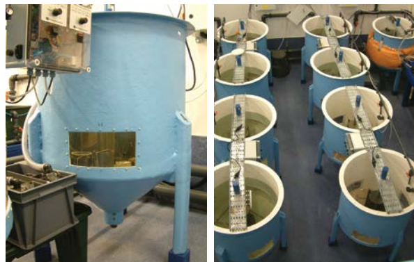
Fig 6.13 Vortex Resuspension tanks (VORTS) used by Last et al. (2011) at the Scottish Association of Marine Science (SAMS) to measure the sensitivity of animals to varying levels of suspended sediment and to burial, © Dr Kim, Last of the Scottish Association for Marine Science.
