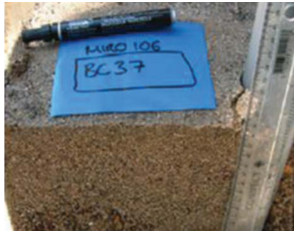
Fig 6.12 A box-core profile showing the structure of the seabed deposits sampled approximately 300m south of an active dredge zone in licence area 430 in the southern North Sea. The sand deposited over the surface of coarser gravel material can be seen. From Newell et al. (2004a).
