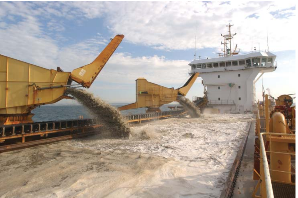
FIGURE 1 A typical modern marine aggregate dredger at work, the 8500t capacity Sand Falcon , operated by CEMEX UK Marine Ltd.
